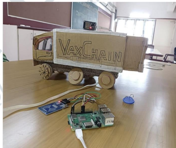
Fig. 2. IOT Setup having temperature sensors and RFID kit
