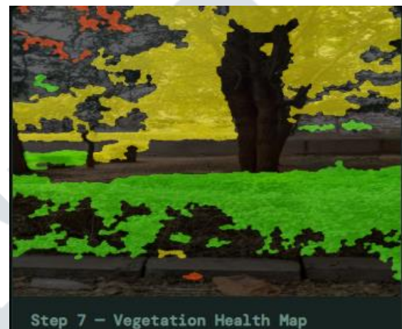
Figure 9. Each patch is classified and displayed as a color-coded map showing vegetation health.
