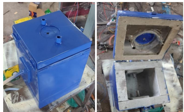
Figure 6. Aging Chamber with Inside View
