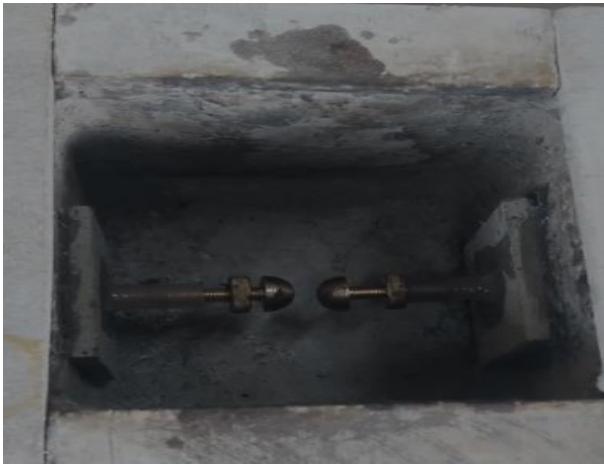
Figure 7. Spherical Rods Inside the Aging Chamber That Will Provide the Pulsed Electric Field
