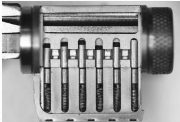
Figure 1: A cutaway pin-tumbler lock (Courtesy of Marc Weber Tobias).
