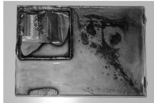
Figure 2: The 4758 partially opened showing (from top left downward) the circuitry, aluminium electromagnetic shielding, tamper sensing mesh and potting material (courtesy of Frank Stajano).
