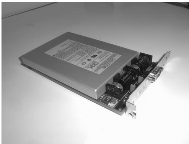
Figure 1: The IBM 4758 cryptoprocessor (courtesy of Steve Weingart).
