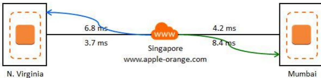
Figure 2: Latency-based Routing: Diagramme showing the overview of the latency-based routing [java point].
